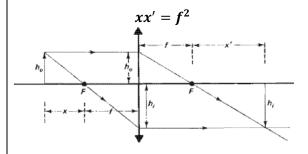
x .- Object distance from Focal Point x .- Image distance Focal Point Focal Distance f
